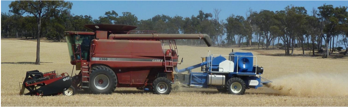
Figure 1.1: Harrington Seed Destructor (HSD) attached to a CASE IH 2388
