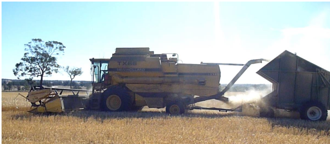
Figure 2.3: Riteway Farming Australia chaff cart attached to a New Holland TX 66 combine harvester
