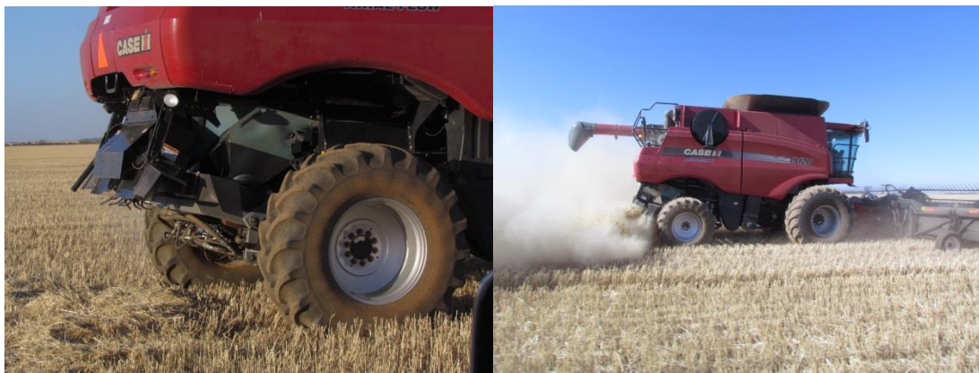
Figure 1.8: a) CASE IH 9120 with two Prototype 1 mills attached (left) b) harvesting wheat at approximately 40 t/h grain throughput (right)
